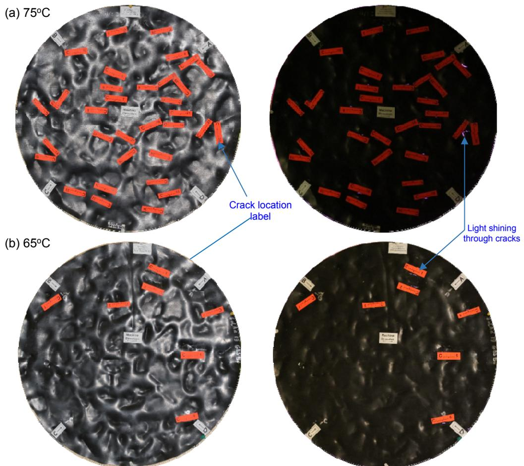
Figure 5. GMB specimens (0.6 m in diameter) after termination of GLLS experiments showing crack locations (marked with red labels) and light shining through some of the larger cracks (fine white lines in the right photograph) at (a) 75°C; (b) 65°C.
