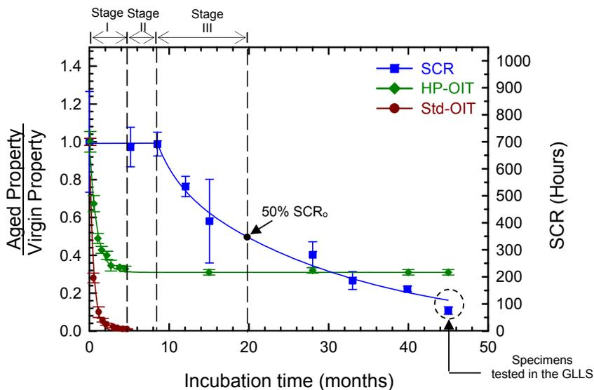
Figure 2. Change in properties with time for the tested GMB immersed in leachate at 85°C.
