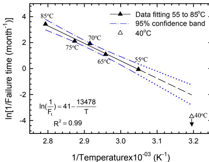
Figure 6. Variation of natural logarithmic of  $1/F_t$  versus  $1/\text{temperature}$  in Kelvin (Arrhenius plot) (modified from Abdelaal et al. 2014).
