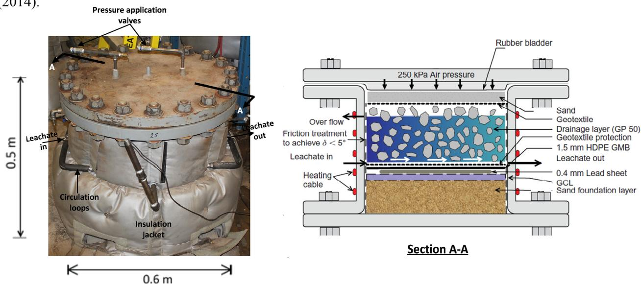
Figure 3. GLLS test Apparatus (modified from Abdelaal et al. 2014).
