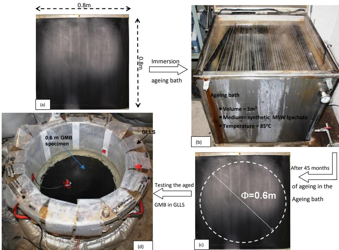
Figure 1. Pre-aging process involving (a) sheets of virgin GMBs 80x80 cm; (b) immersion of the sheets into ageing baths in MSW leachate at 85°C for 45 months; (c) after ageing and reaching the desired SCR; (d) testing aged GMB in GLLS under simulated landfill liner configurations.
