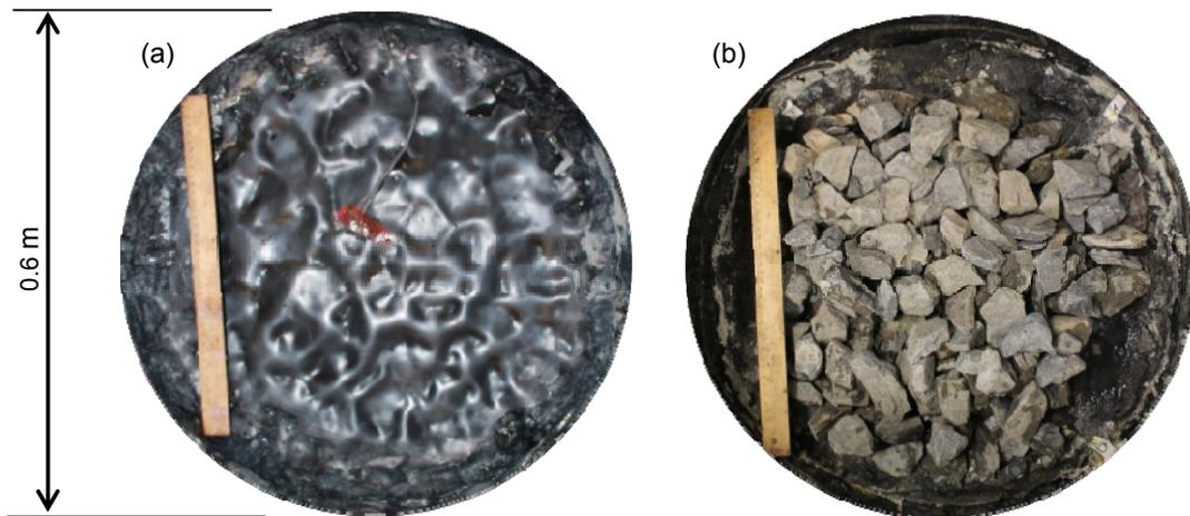
Figure 4. GMB specimens (0.6 m in diameter) from 40°C GLLS experiments after 4 years of testing showing a) intact GMB specimens; b) drainage layer in contact with the GMB in the GLLS. Scale is 40 cm in length.
